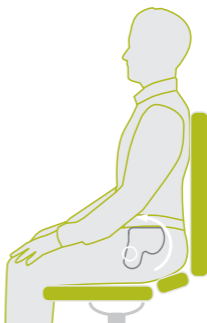
Sitzkeil-Effekt Seat-wedge effect Wig-effect Effet de coin de siege
